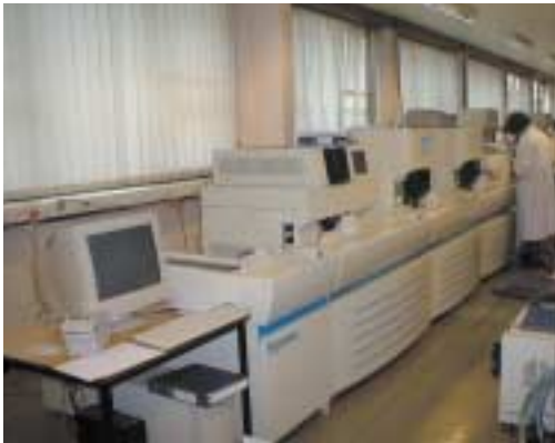
Part of the first phase of the Walsgrave installation showing the HST system: the film maker and two haematology analysers.
